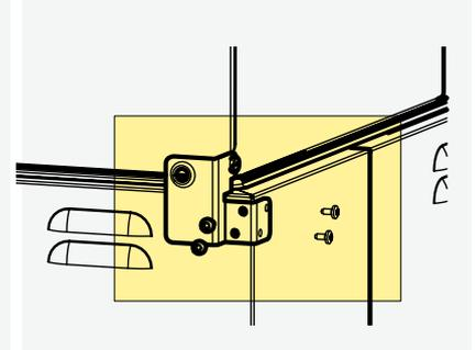
4. Tighten screws and check that the lid fits tightly.
